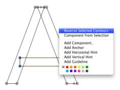
For interpolation, path order, starting points and path directions need to be compatible and consistent throughout all font masters. For more details on interpolation, see chapter 9, 'Multiple Master' (p. 73).
