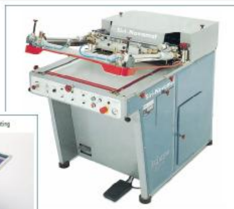
Fig. 2.4-14 Semi-automatic screen printing machine for printing on flat substrates (Siri/Oschonow)
