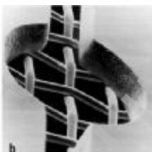
a Direct stencil; b Direct/indirect stencil
