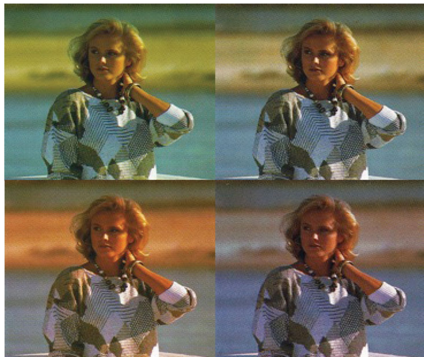
This portion of one of the Linotype-Hell test images shows the wide colour variation from four of the eight test sequences. Clockwise from the top left, 4:MCYK, 5:MYCK, 6:YCMK, 8:CMKY
