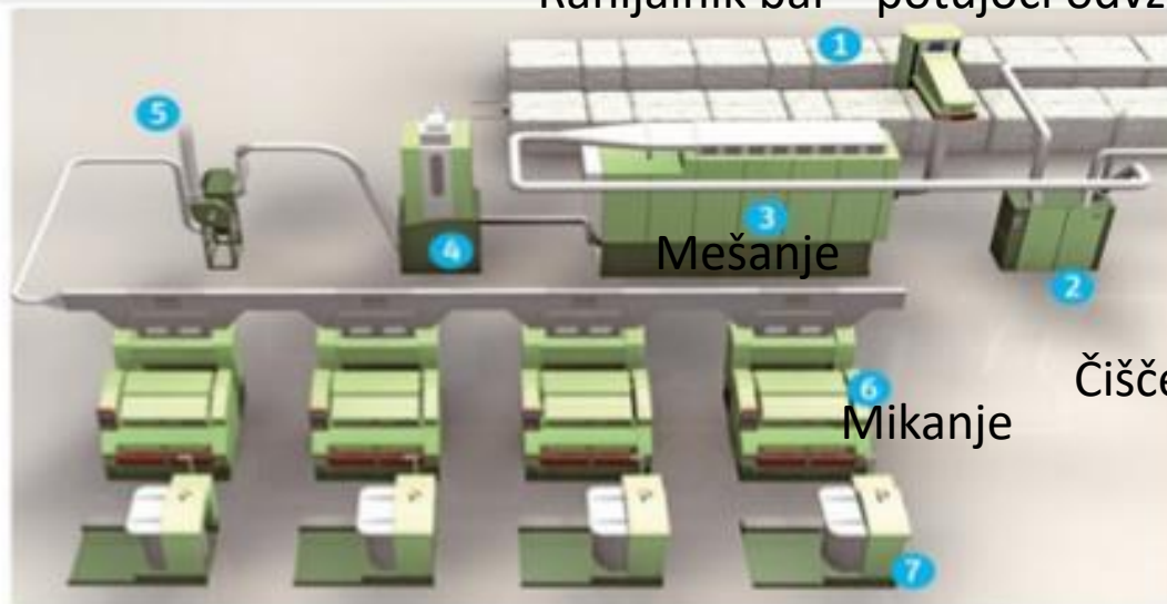
Figure – Rieter blowroom line; 1. Bale opener UNIfloc A11; 2. Pre-cleaner UNClean B 12; 3. Homogenous mixer UNImix B 75; 4. Storage and feeding machine UNIstore A 78; 5. Condenser A 21; 6. Card C 60; 7. Sliver Coiler CBA 4
