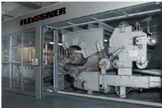
Fleissner AquaJet of 3.6 m working width for polyester and polyester blends of medium and heavy weight. The line consists of opening, card, crosslapper, AquaJet, dryer, winder. Applications are multipurpose such as automotive, filtration and others.
