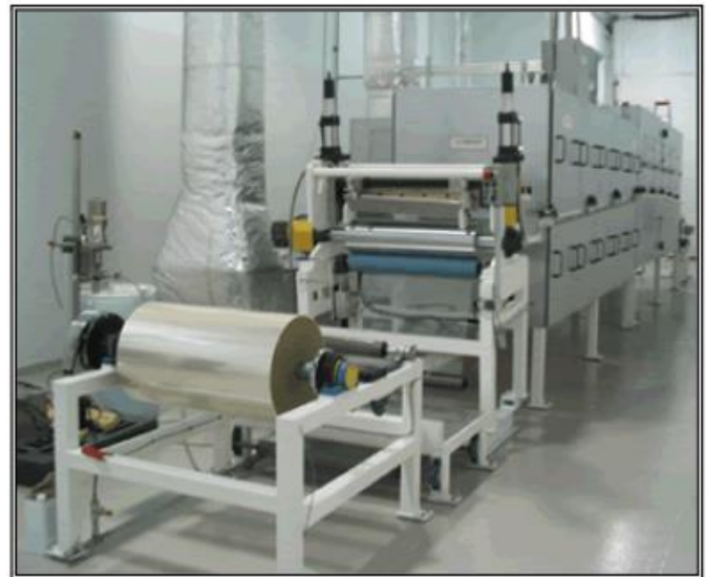
Infrared Air & Hot Air Dryer on a Coating Line
