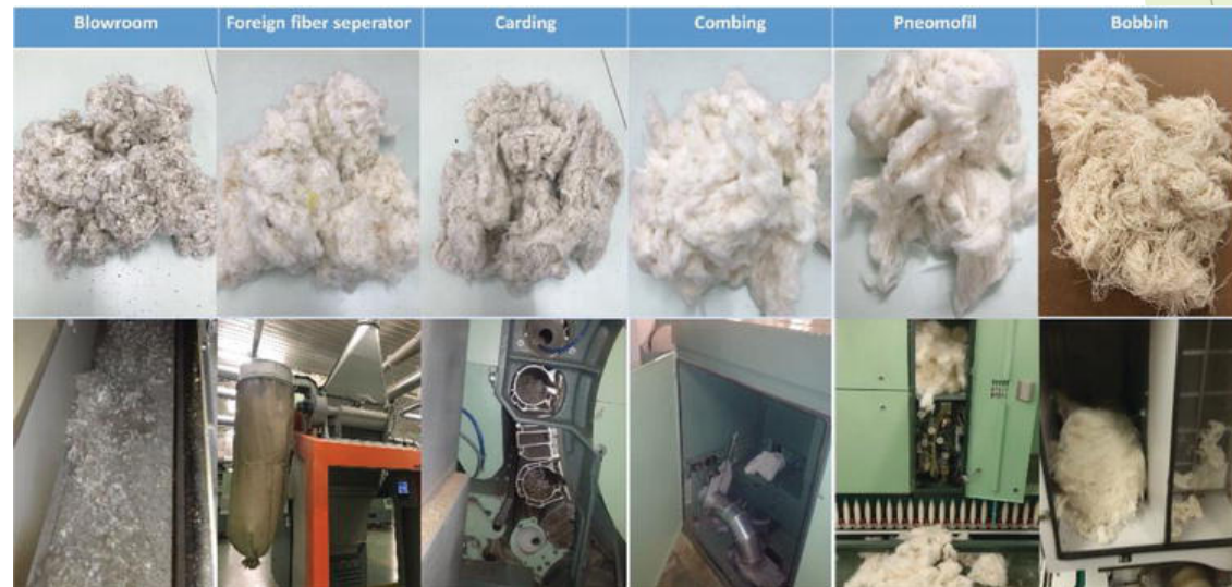
Figure 3. Spinning wastes and their sources 13
