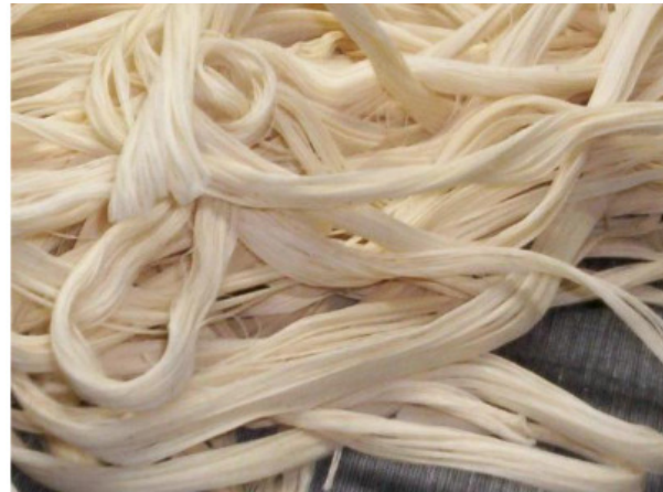
Figure 4. Warp sheet wasted during sizing 14
