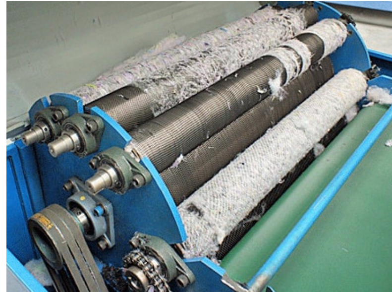
Figure 4. Shredding machine rotation drums with metal pins. 1
