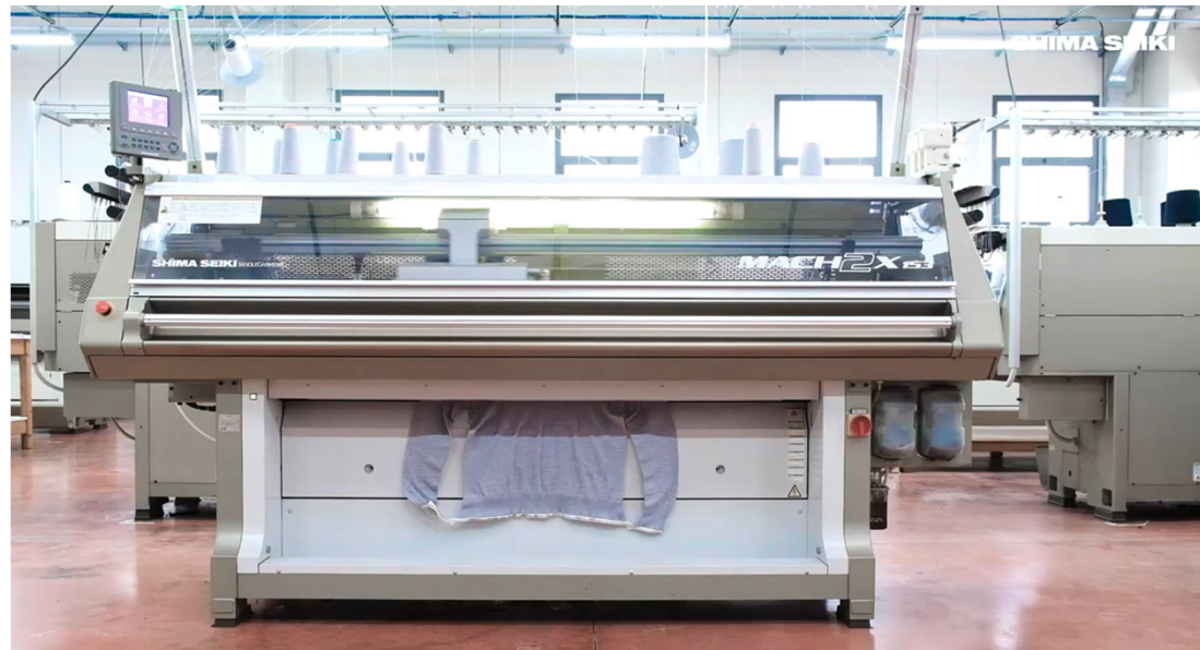
Figure 33. Shima Seiki's Wholegarment® knitting on MACH2X 153 machine 14
