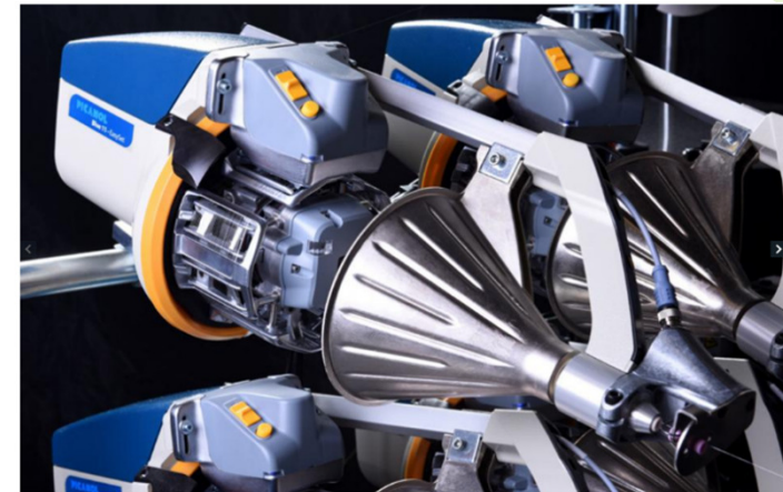
Figure 10. Blue prewinders by Picanol 7
