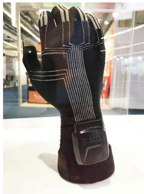
Figure 30. A knitted augmented and virtual reality sensor glove from Stoll 12
