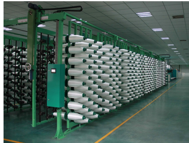
Figure 13. Modern creel for beam manufacturing 10
