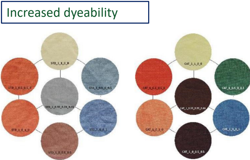
Figure 21. Colour of untreated (left) and cationised (right) cotton dyed with vat dyes 25
