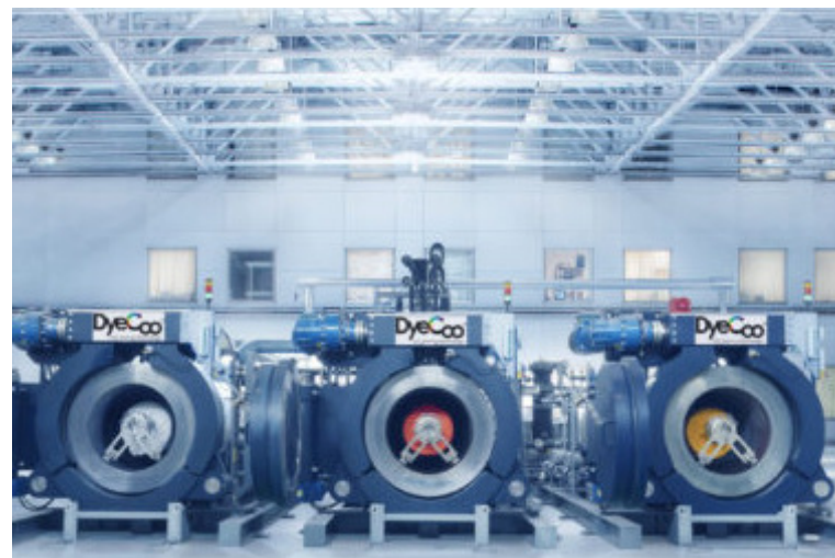
Figure 23. Dyeing PES in CO 2 27
