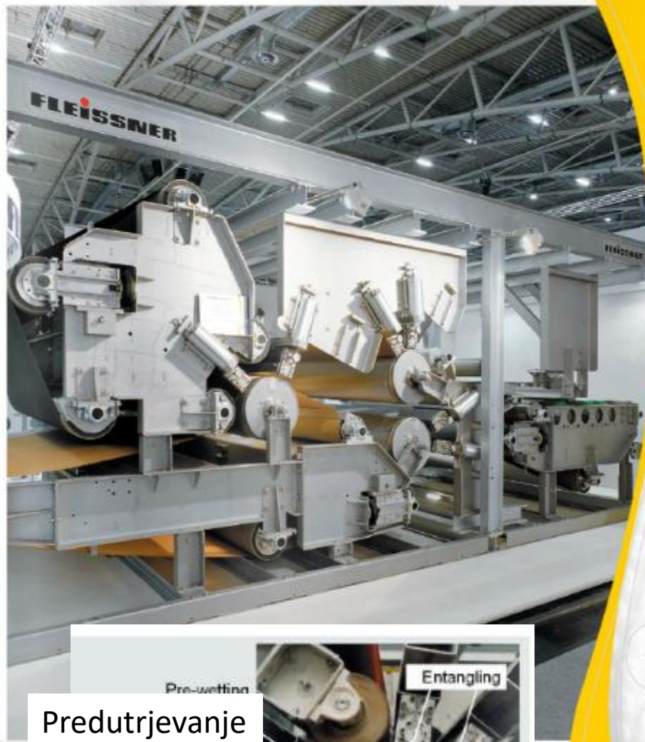
Fleissner AquaJet of 3.6 m working width for polyester and polyester blends of medium and heavy weight. The line consists of opening, card, crosslapper, AquaJet, dryer, winder. Applications are multipurpose such as automotive, filtration and others.
